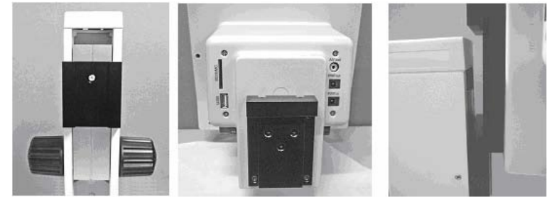
The dove-tail groove on trestle
